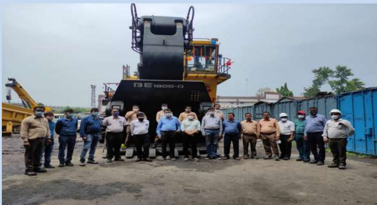
Hydraulic Shovel HS-37 with frontload bucket capacity of 12.2 Cum introduced at Rajmahal
